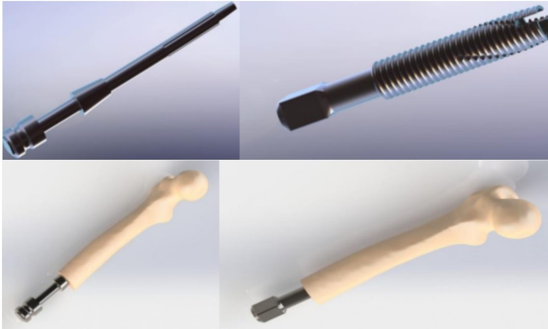
Fig. II: Left: OPL (Osseointegrated Prosthetic Limb), Right: OPRA (Osseointegrated Prostheses for the Rehabilitation of Amputees) [Adopted from: Mirulla AI, Di Paolo S, Di Simone F, Ingrassia T, Nigrelli V, Zaffagnini S, et al. Biomechanical Analysis of Two Types of Osseointegrated Transfemoral Prosthesis. Applied Sciences . 2020; 10(22):8263. https://doi.org/10.3390/app10228263 ] 10
